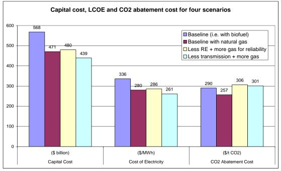
Figure 7 compares the capital cost and cost of electricity for the 'copper-plate' additions to the transmission system (Scenarios 1, 2 and 3) and the scenario with reduced additions to the transmission system (Scenario 4).
