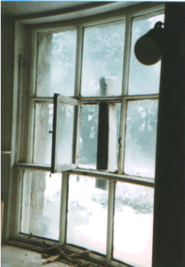
Plate 1. The light metal box, placed in the north window of the Eastern Tower at Armagh Observatory which contained the ‘external’ and maximum and minimum thermometers prior to their removal to a Stevenson Screen in 1885. The hinged central pane of the upper window sash allows access to the thermometers from an inside staircase. Adjacent buildings were unheated at the time.
